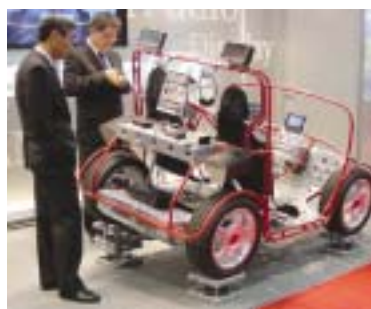
The Yazaki data network architecture buggy demonstrates streaming audio and video over a vehicle optical fiber network.
