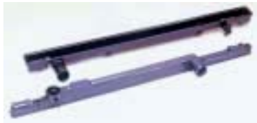
Radiator end tanks were the subject of recycling tests conducted by Denso.
