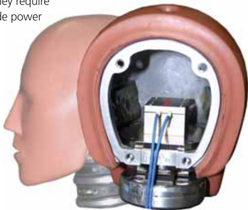
Data acquisition modules from Messring are small enough to fit inside the robot, sending data out via a single wire.
