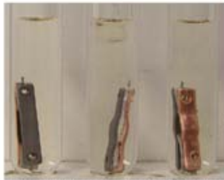
Figure 2. Photograph of Sealed Tubes After Aging at 150°C for 24 hr
