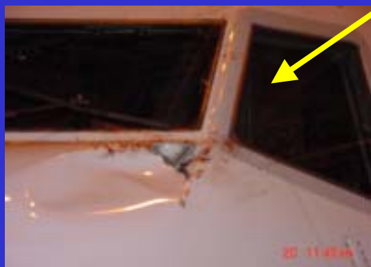
Snow goose penetration into cockpit, B-727, Memphis, Nov 2001
