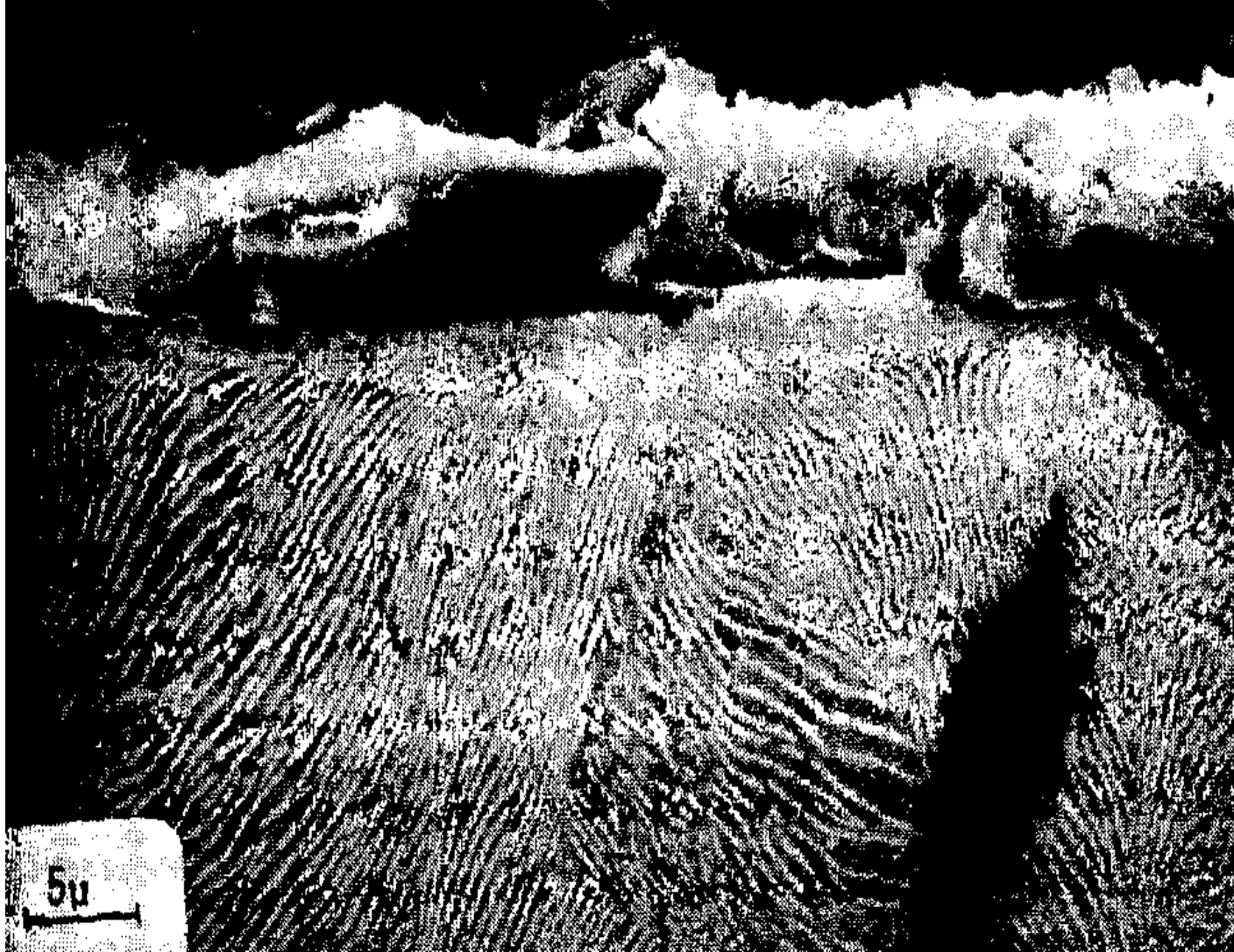
SEM micrograph of the cross-section of cast iron drum. It shows transfer film and deformed cementite platelets in the cast iron subsurface structure.
