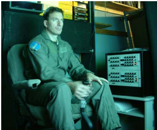
Figure 1: STI Simulator with McFadden Control Loader and Projected Display
