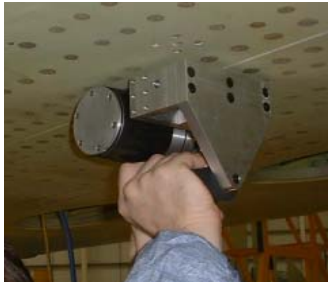
Ultrasonic Wheel Array Sensor Instrument (NDT Solutions Ltd.)
