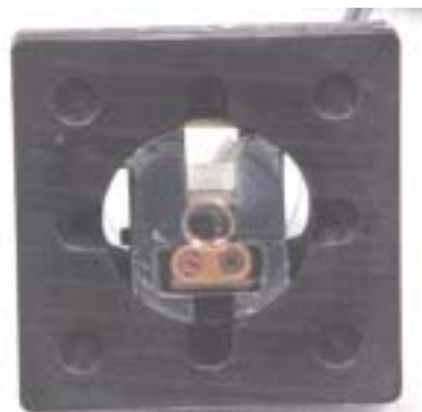
Bottom of probe showing two coils
