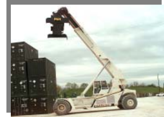
RTCH Kalmar Contractor
