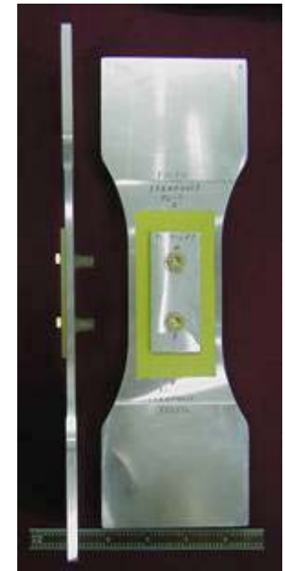
8% Effective load Transfer dogbone specimen
