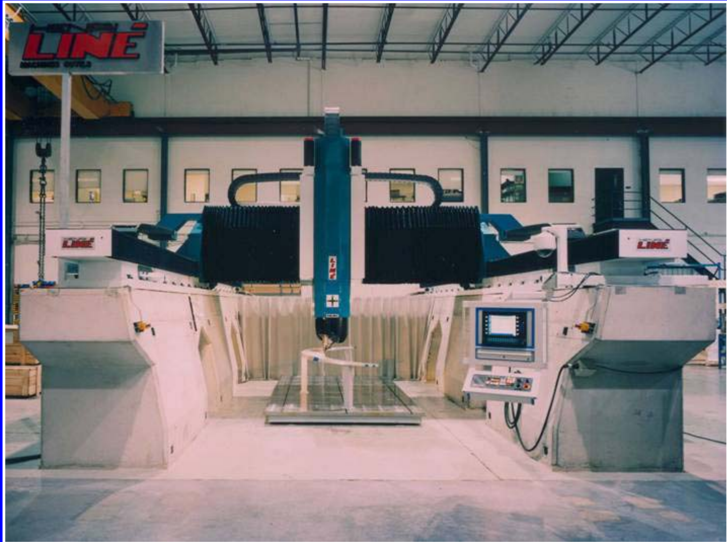
SU-15 High speed machine equipped with Linear motors
