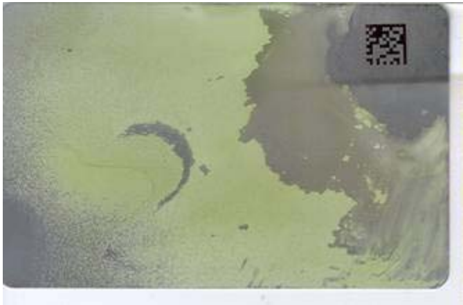
Laser Bonding after 24 hrs in paint stripper.
