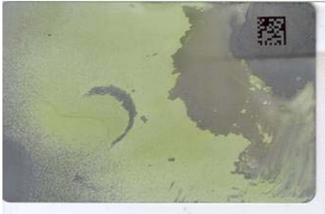
**Laser Bonding after 24 hrs in paint stripper.**
