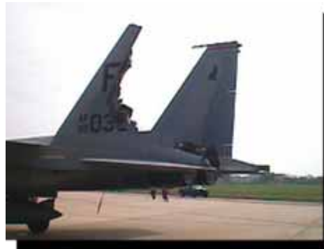
F-15 Vertical Failure
