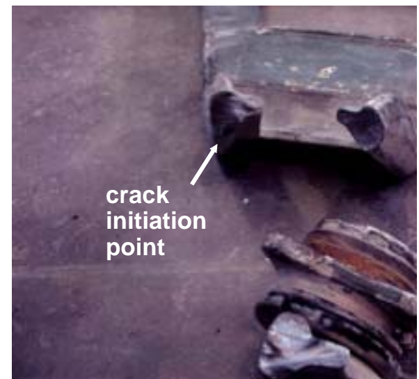
Fatigue failure simulations for three terrains (10HR, 6WB & BB) identified hot spot at the same location.
