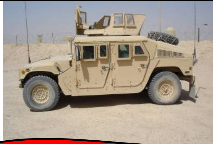
Improved door with rocker panel upgrade highlighted
