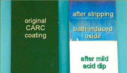
The fast and thorough stripping of CARC via molten salt is a prime example of the efficiencies of these extreme processes.
