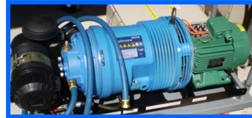
Electric Air Compressor
