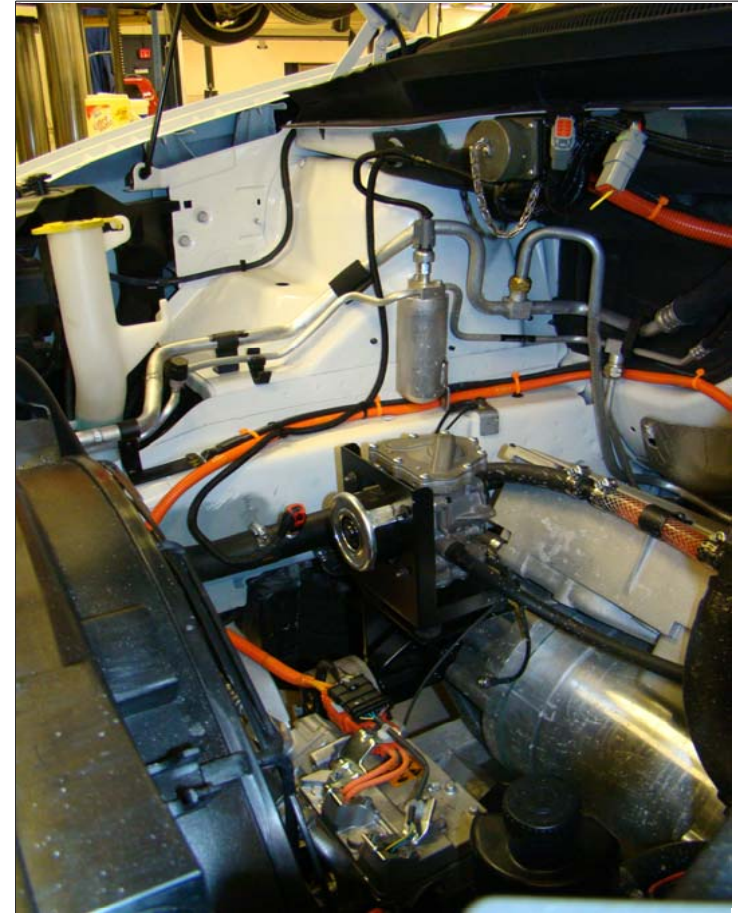
Engine compartment with 150kW Electric Powertrain Module
