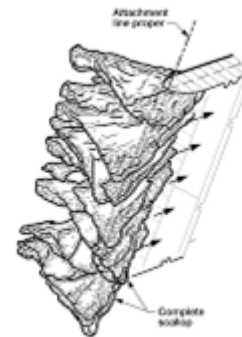
The feathers join along the preferred direction of growth to form ridges. The ridges join to form scallop tips
