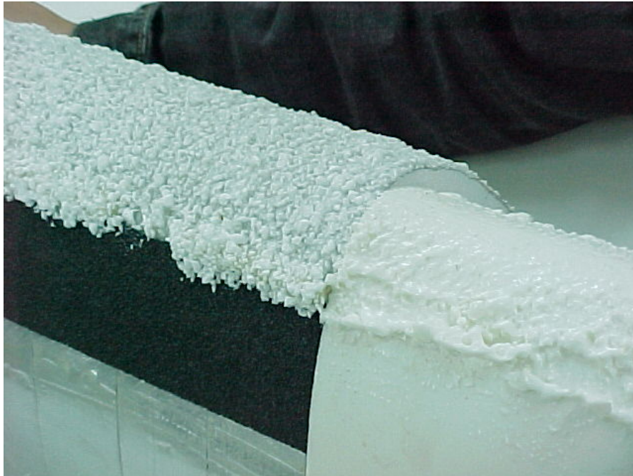
SIMULATED ICE SHAPE (Left side of pictures) VS FAA MOLDS (Run 5/6 - LOWER SURFACE)
