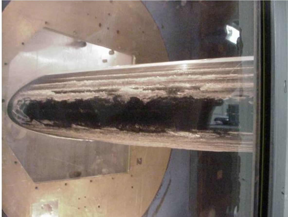
HYBRID MODEL INSTALLED IN THE BF GOODRICH TUNNEL
