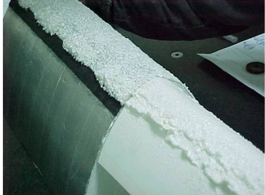
SIMULATED ICE SHAPE (Left side of pictures) VS FAA MOLDS (Run 5/6 - UPPER SURFACE)
