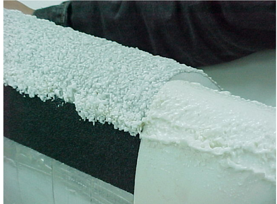
SIMULATED ICE SHAPE (Left side of pictures) VS FAA MOLDS (Run 5/6 - LOWER SURFACE)
