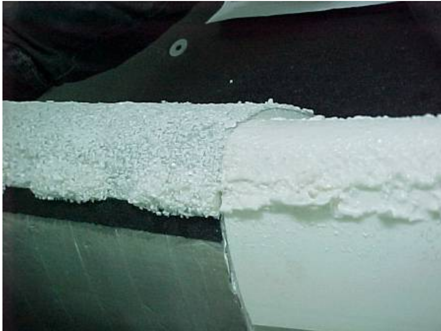
SIMULATED ICE SHAPE (Left side of pictures) VS FAA MOLDS (Run 5/6 - UPPER SURFACE)
