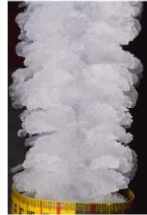
Complete scallop, d_{cr} = 0 \text{ mm}
