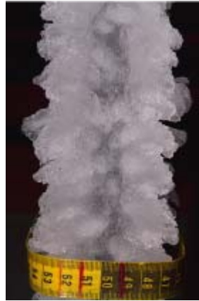
Incomplete Scallop, d_{cr} = 5 \text{ mm}
