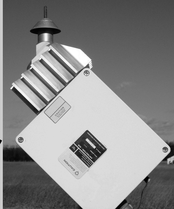
Freezing Rain sensor (Goodrich)
