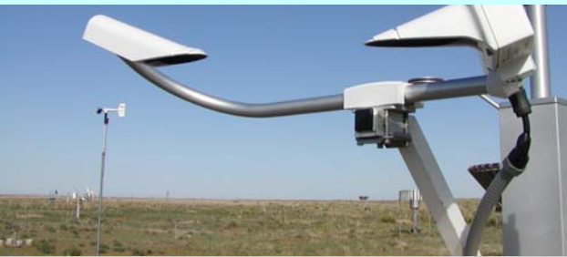
Precipitation Type sensor (Vaisala PWD-22) EPI sensor
