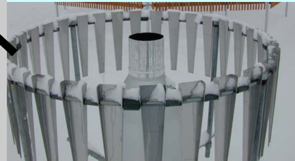
Weighing Snowgauge (GEONOR)
