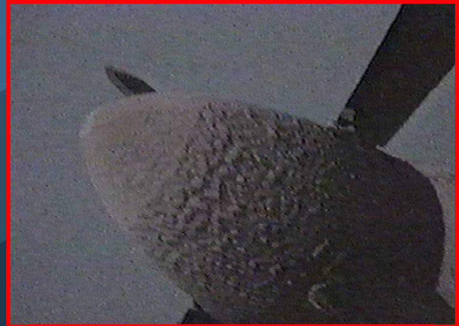
Ice accretion on the spinner under SLD's
