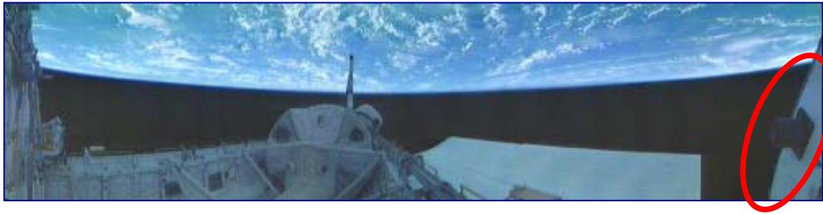
**REALITY:** Seams in insulation blanket inside payload bay
