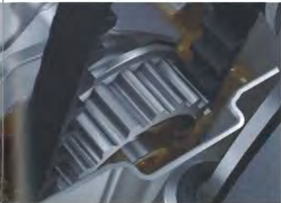
Ford EcoBoost 1.0 litre gasoline engine, with timing belt running in oil. Source: Ford youtube.com video.
