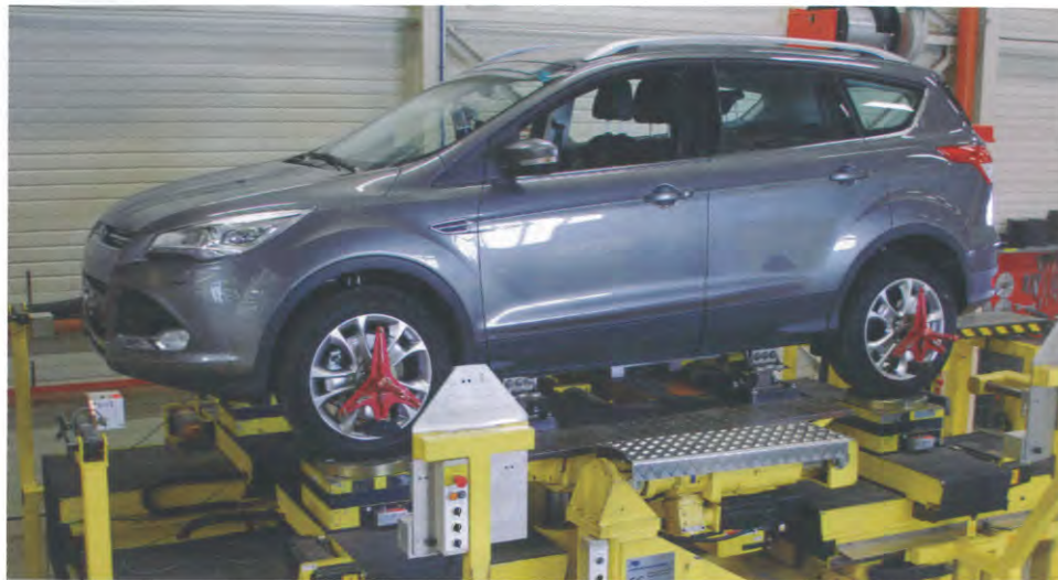
Ford's Anthony Best Dynamics steering rig at its Lommel facility
