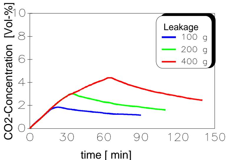
**Figure 1** CO<sub>2</sub> concentration in a vehicle cabin with different CO<sub>2</sub> charges for a simulated evaporator leakage, Vol.-flow is 200 litre/hr, 100 % recirc.
