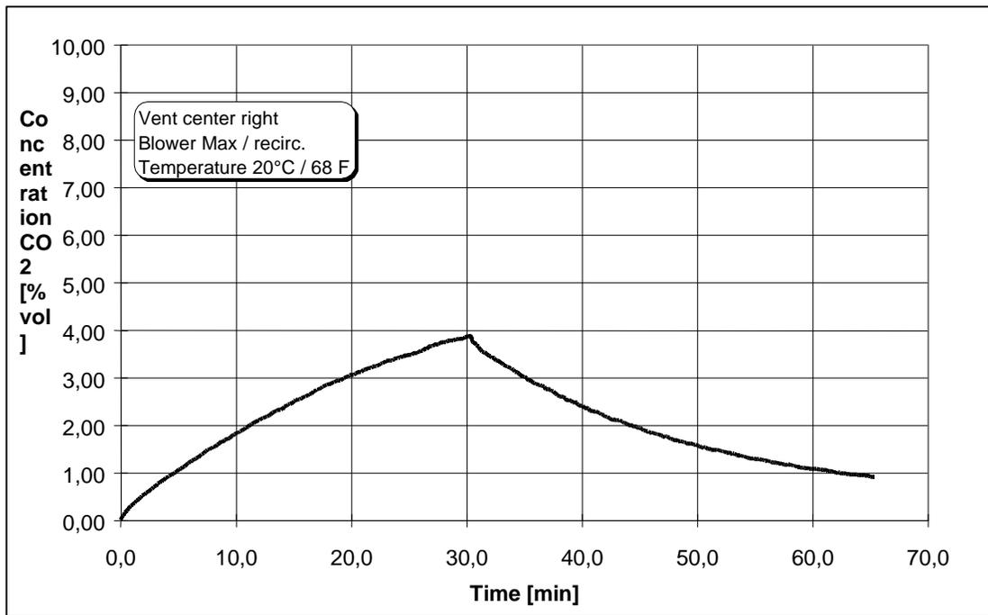
**Figure 3:** Experimental results of a continuous release of 500 g CO<sub>2</sub> with 500 l/h into the passenger compartment of midsize vehicle.
