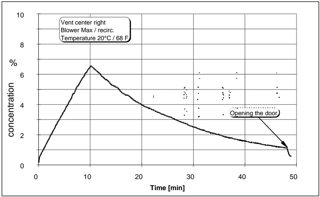
**Figure 2:** Experimental results of a continuous release of 500 g CO<sub>2</sub> with 1500 l/h into the passenger compartment of a midsize vehicle.
