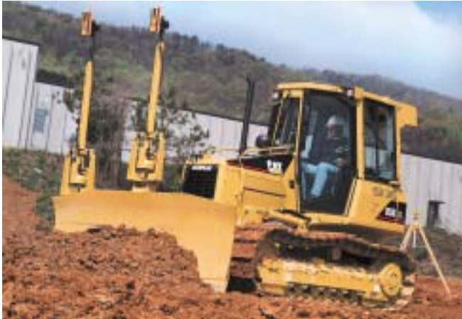
The Caterpillar G-Series tractors are designed for construction applications requiring maneuverability and controllability when dozing, grading, cutting ditches, backfilling ditches, spreading fill, and landscaping.
