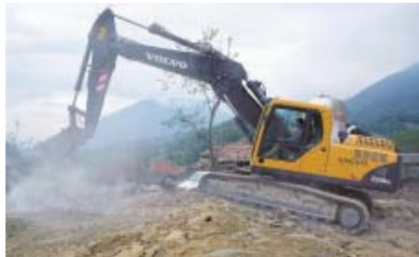
The Volvo EC210B NLC excavator has a transport width of 2.54 m (8.3 ft) for easier access to hard-to-reach job sites.
