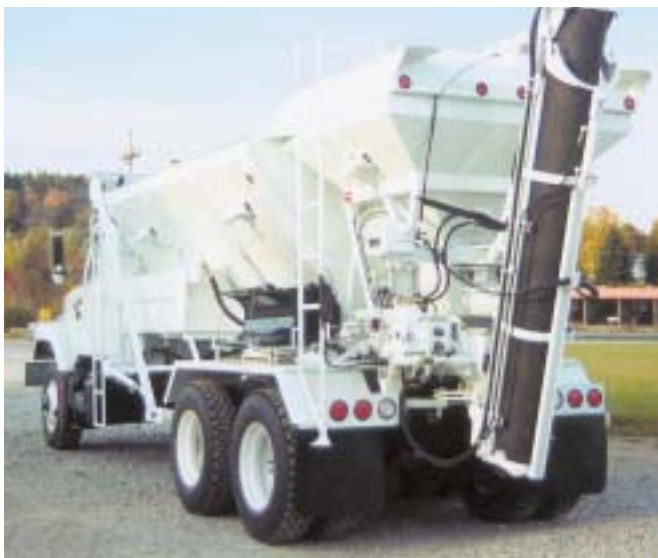
Elkin mobile mixers are custom designed and sized to fit either existing or new truck chassis and are available in a wide range of rear-discharge, front-discharge, and trailer or skid-mounted configurations.
