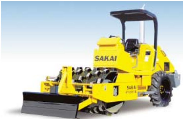
The Sakai SV201TB soil compactor is powered by a Cummins diesel engine that delivers 60 hp (45 kW).
