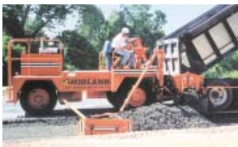
Midland's Millennium wideners include curved spreader blade sections for added strength and smoother finishes during placement of material.
