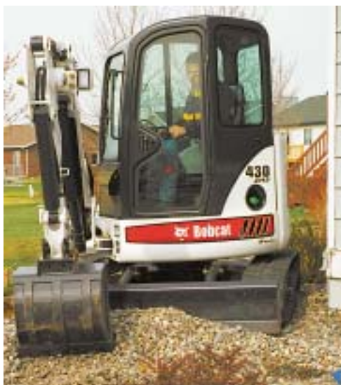
The Bobcat 430 compact excavator has zero house swing and can travel at up to 5 mph (8 km/h).
