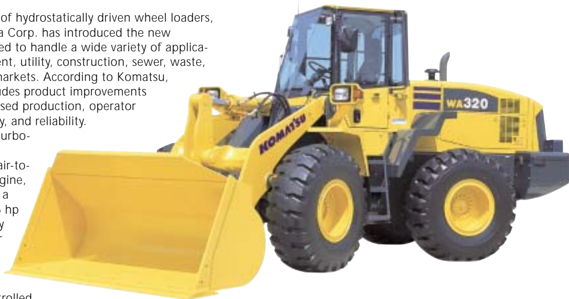
The WA320-5 wheel loader from Komatsu has a turbocharged diesel engine that produces 166 hp (124 kW), and features an electronically controlled hydrostatic transmission.
