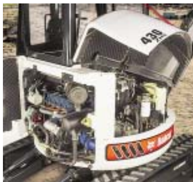
A direct-injection, turbocharged Kubota engine delivering 43 hp (32 kW) powers the Bobcat 430 ZHS excavator.
