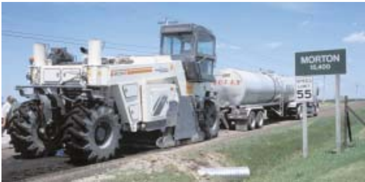
The Wirtgen WR 2500 S road reclaimer from Wirtgen America features an upgraded Mercedes V12 diesel engine.
