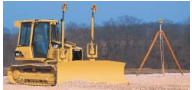
An optional feature on all Caterpillar track-type tractors is the AccuGrade system, which features laser receivers mounted on the blade. An off-board transmitter emits a 360° reference beam, and the receiver can automatically control the machine's hydraulic system to adjust blade lift and tilt as the machine moves over the area.
