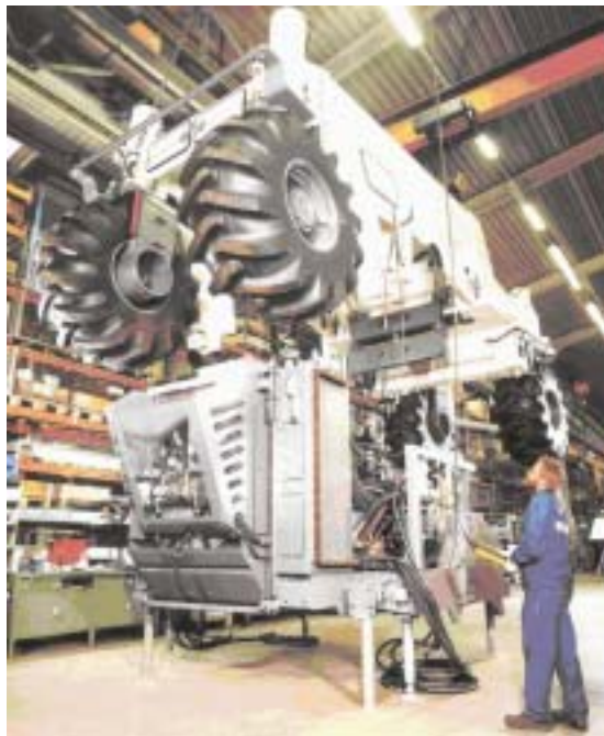
After the engine is mounted on its frame with pumps and radiator fitted, the entire WR 2500 S stabilizer chassis is lowered into place.
