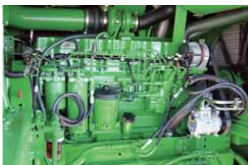
The Deere 9996 cotton picker is powered by a 350-hp (261-kW), 8.1-L PowerTech Tier II compliant engine (below).
