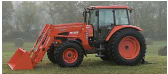
A single-lever joystick operates the front loader on the Kubota M125X, which has a mechanical self-leveling linkage.
