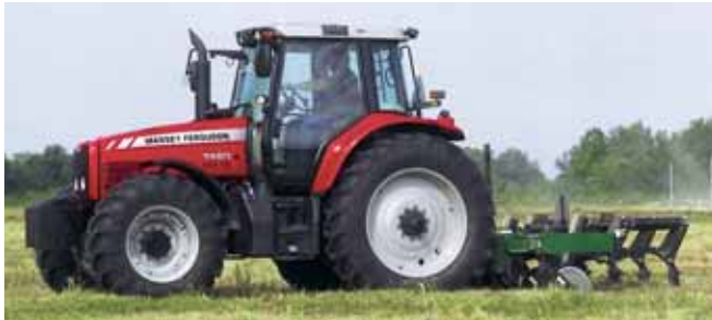
The Massey Ferguson 7400-series tractors have separate oil reservoirs for transmission and auxiliary hydraulics.
