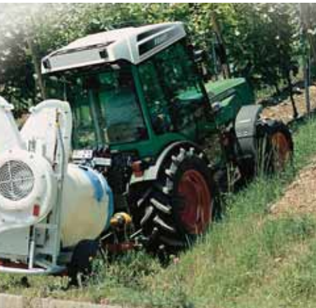
The new 200 Series tractors from Fendt have front-, mid-, and rear-mount options, electrohydraulic control of up to six spool valves, and a three-point hitch system.
