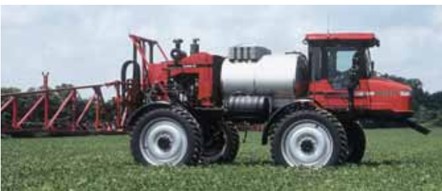
By moving the engine to the rear and the product tank to the middle, the new Case IH SPX3310 Patriot sprayer achieves an almost equal weight distribution for a more balanced footprint in the field.
