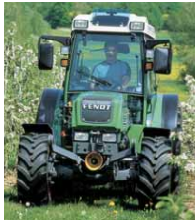
Fendt 200 Series tractors have road speeds as high as 25 mph (40 km/h) and creeper gears for speeds as low as 0.18 mph (0.3 km/h).
