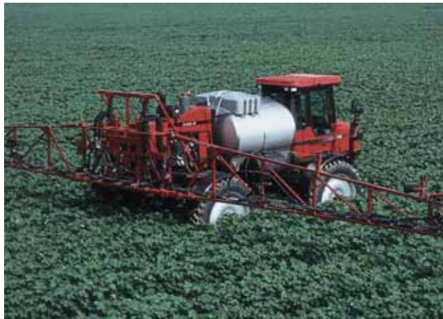
The new Case IH SPX3310 offers adjustable 60/80- or 60/90-ft (18.3/24.4- or 18.3/27.4-m) booms in five- or six-section configurations.
