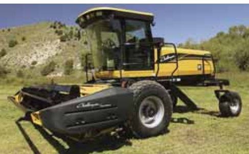
B-series windrowers from Challenger have a computer that tells the tractor which header is attached when the electrical wiring harness is connected, and hydraulic flow to the drive motor automatically adjusts to match drive-speed requirements.
