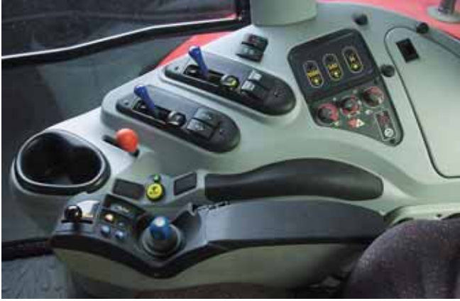
Electronic Engine Management and Remote Valve Management System are at the operator's fingertips in the new Massey Ferguson 7400-series tractor cab.
