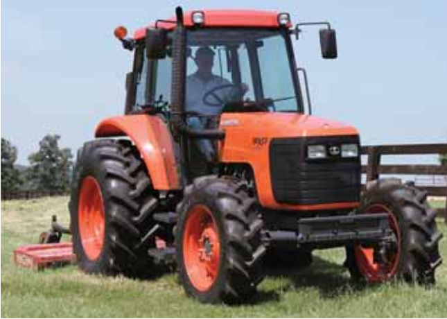
The M955 utility tractor from Kubota comes standard with a fully synchronized main and hydraulic shuttle transmission with Swing Shift or Swing Shift Plus.
