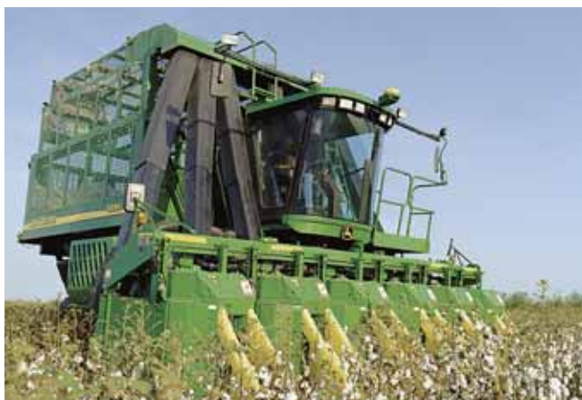
The Deere 9996 cotton picker is powered by a 350-hp (261-kW), 8.1-L PowerTech Tier II compliant engine (below).
