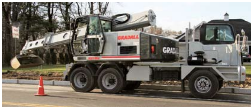
Gradall's new XL 5100 III excavator features a simplified yet more efficient powertrain and a shorter carrier for easier mobility.
