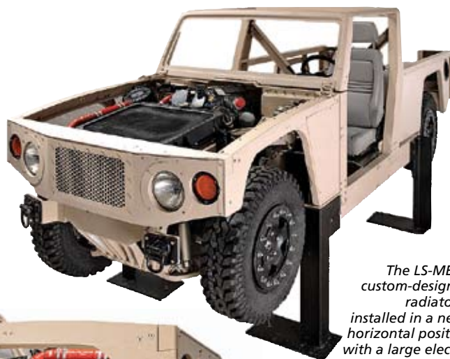
The Zeus Light Strike Medical Evacuation Vehicle is designed to fit within the cargo compartment of the V-22 Osprey vertical takeoff and landing aircraft.
