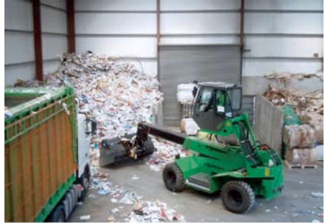
The 305 Multihandler's bucket and extendible arm give the operator additional reach into a pile.
