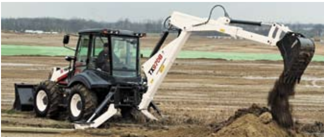
The TX970B offers all-wheel steer, including crab steer, as well as a long backhoe boom for increased, 24-ft (7.3-m) reach and 20.3-ft (6.2-m) digging depth.
