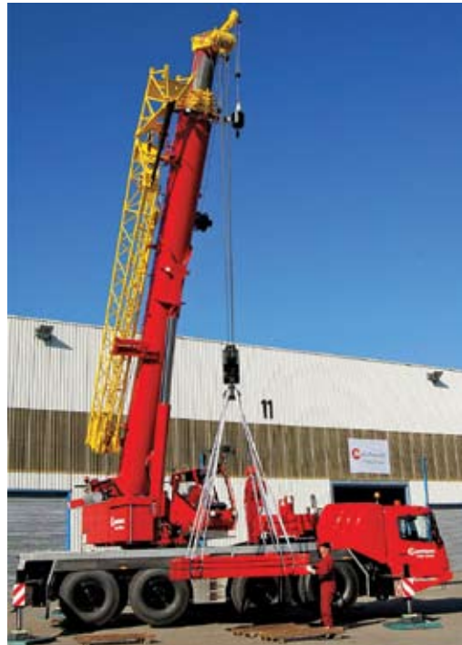
The Grove GMK4100, Manitowoc Crane Group's newest all-terrain crane, offers an extendable 52-m (171-ft) boom and sleek new operator cab.
