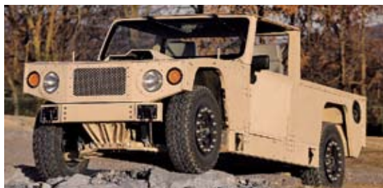
The Zeus Light Strike Medical Evacuation Vehicle is designed to fit within the cargo compartment of the V-22 Osprey vertical takeoff and landing aircraft.
