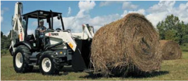
Terex's TX760B loader backhoe is powered by a 4.4-L 86-hp (64-kW) Perkins turbo induction engine.
