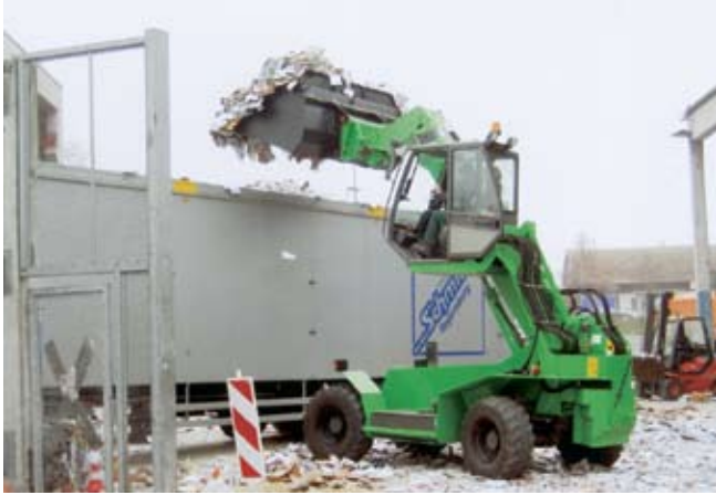
The hi-rise cab on the 305 Multihandler provides an eye-level view of 13.3 ft (4.1 m) and gives the operator a clear view of where the load is going.
