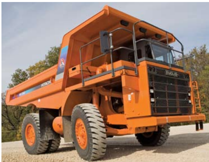
The EH750-3 (above) is powered by an inline six-cylinder Detroit Diesel engine, while the EH1100-3 uses an MTU Detroit Diesel 12 V series 2000 diesel engine.
