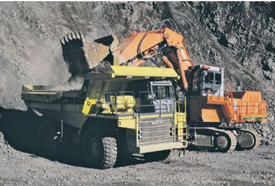
Like the EH750, the EH1100 rigid dump truck (above) offers a low loading height and large target area to facilitate easy, quick loading by a variety of loading tools.
