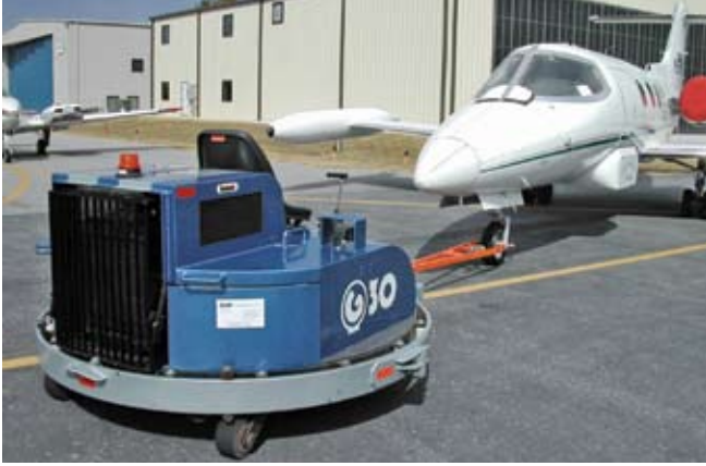
Model G-30 omni-directional vehicles are being used at Warner Robins to assist in aircraft maintenance operations.
