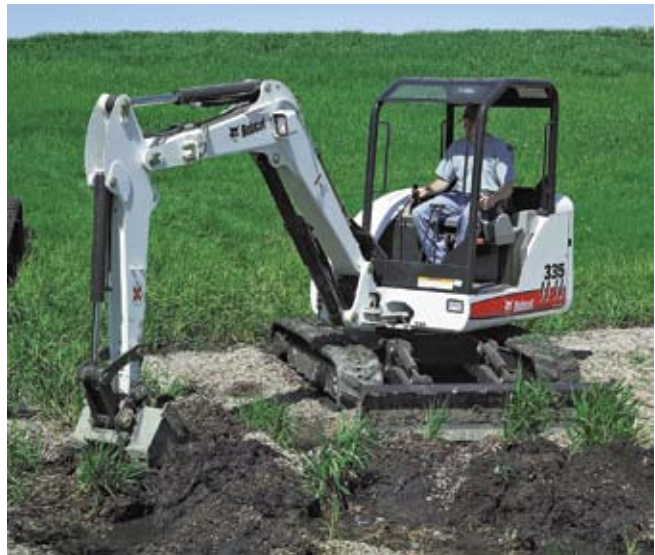
The 335 compact excavator delivers 5262 lb (23.4 kN) of arm breakout force and 7892 lb (35.1 kN) of bucket breakout force from its compact, 70-in (1780-mm) track width.
