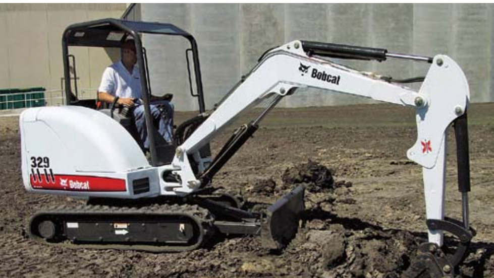
Bobcat's new entry-level 329 compact excavator features a torque-limiting dual-outlet piston pump that provides smooth, predictable hydraulic control.
