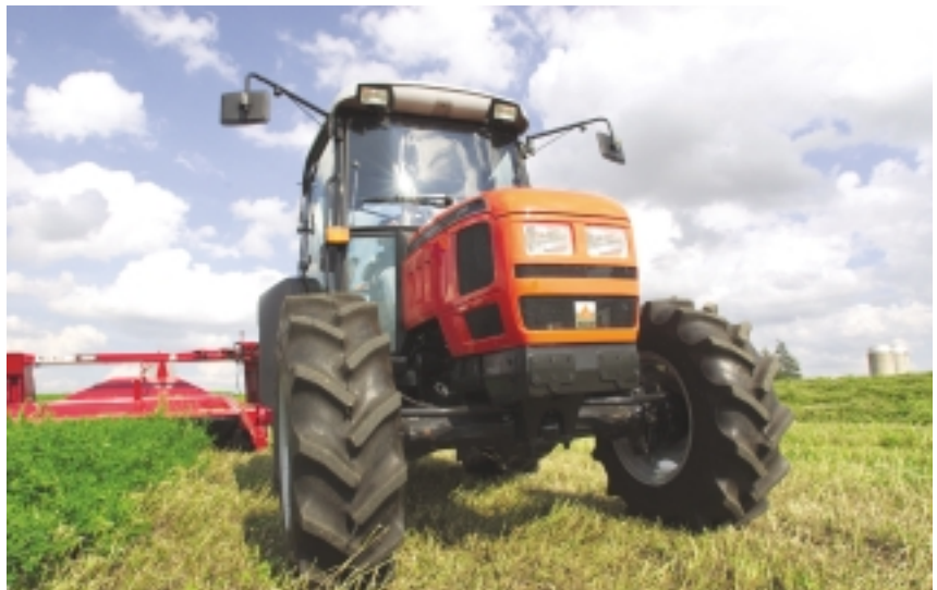
AGCO GT tractors have a turning radius of 10.5 ft (3.2 m).
