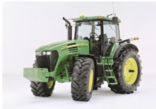
The Deere 7920, rated at 170-hp (127-kW) PTO, is the most powerful 7000 series tractor ever built.
