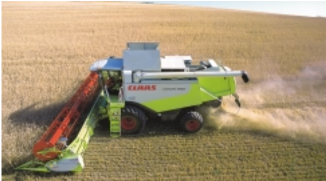
The power of the Claas Lexion 580 increased from 412 to 430 hp (307 to 320 kW) compared to the 480 it replaces.
