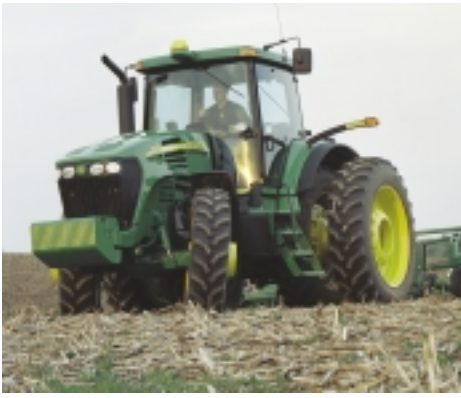
The sculptured-frame design of the Deere 7020 tractors allows the front wheels to tuck under the tractor for an improved turning radius at narrow tread settings.
