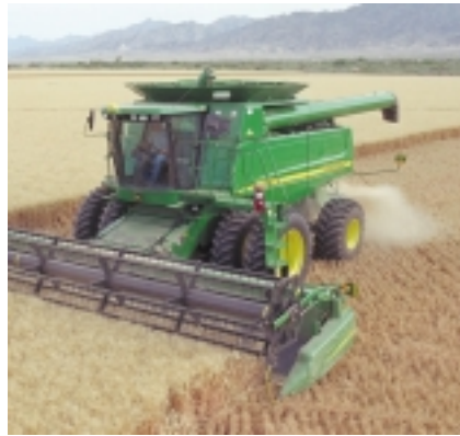
The new 60 Series Combines are powered by 6.8-L, 8.1-L, or 12.5-L John Deere PowerTech engines.
