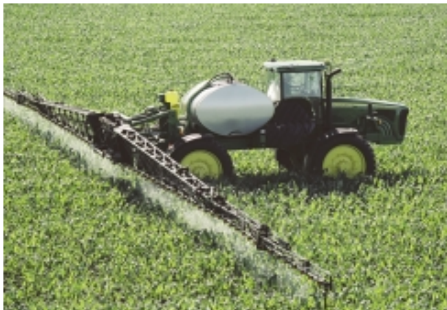
The Deere 4920 self-propelled sprayer comes with a 120-ft (36.6-m) boom.
