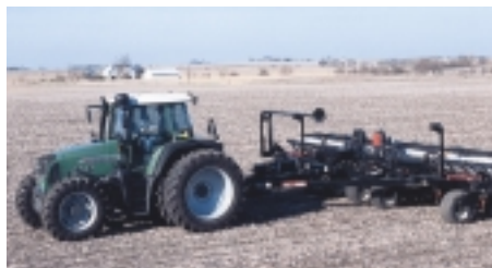
The Fendt 818 Series delivers 160-hp (119-kW), and an intelligent Tractor Management System (TMS).
