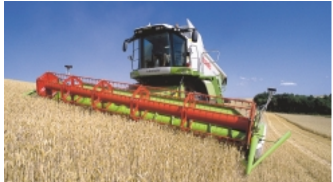
The rotary technology in the Claas Lexion Montana automatically compensates for lateral gradients up to 17%.
