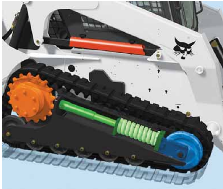
Bobcat's updated K-Series compact track loaders (T180 through T300) feature an additional roller in the track undercarriage for better ride quality and improved service life.
