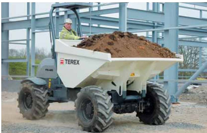
The new PS6-AWS dumper from Terex is powered by an 80-hp (60-kW) Perkins 1100 series diesel engine.
