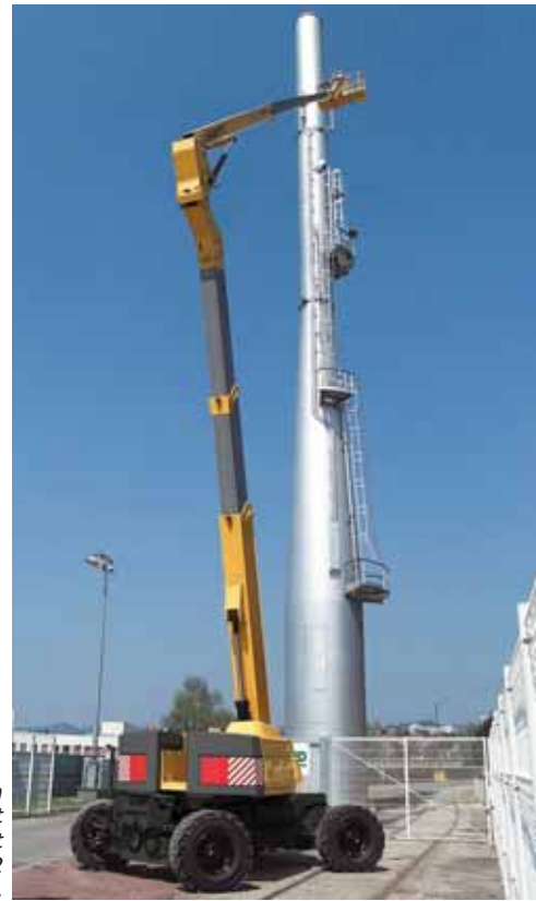
Haulotte's HA 41 PX is a 41-m (134.5-ft) boom lift with an articulation point at 16.5 m (54 ft) and a 19.2 m (63 ft) outreach.
