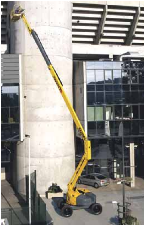
The HA 260 PX diesel articulated boom lift from Haulotte has a maximum working height of 26 m (85 ft) and a maximum horizontal reach of 16.2 m (53 ft).
