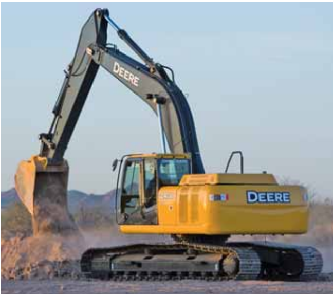
The 240D LC excavator from John Deere is powered by a 6068H turbocharged diesel engine that delivers 177 hp (132 kW).
