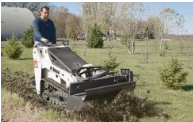
Fifteen different attachments are available for the MT52 mini loader, including the Bobcat tiller.
