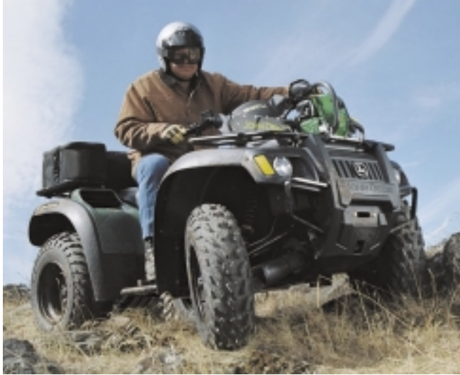
The Deere utility ATV models all feature a progressively locking all-wheel-drive system, hydraulic disc brakes, and four-stroke Rotax engines.
