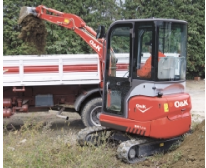
O&K also has a new range of mini-excavators that include variable-displacement pumps for fast and simultaneous movements.
