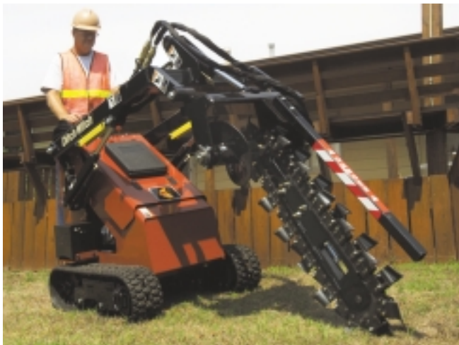
The Ditch Witch SK300 is a track-mounted, stand-on platform skid steer powered by a 13-hp (10-kW) Honda engine.
