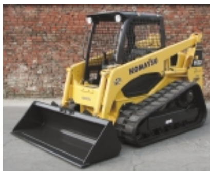
The CK1122-5 is a prototype of a new crawler-type skid-steer loader from Komatsu, with good traction and stability but lower ground pressure than similar wheeled loaders.
