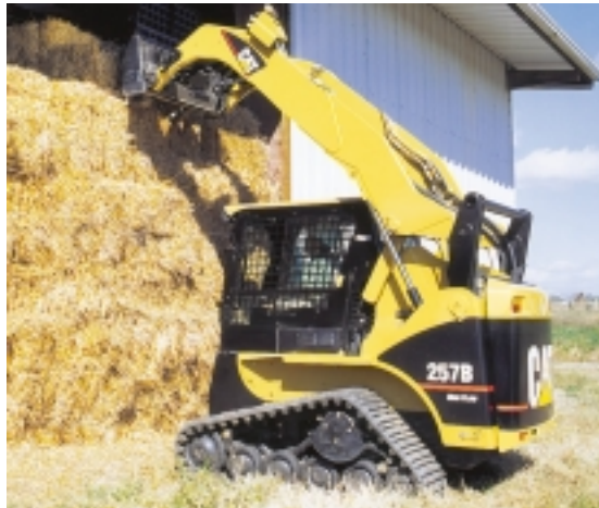
The 257B loader from Caterpillar is powered by the 57-hp (42-kW) Cat 3024C T engine, and has rubber-tracks that combine the technology of the Cat skid-steer loaders with a suspended track undercarriage.
