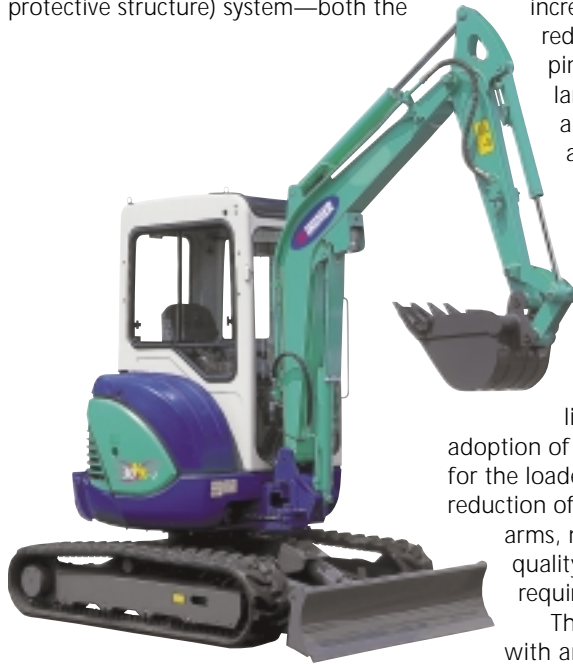
The 30NX-2 mini-excavator from IHIMER is powered by an 18-kW (24-hp), 1.5-L Yanmar low-emissions diesel engine.
