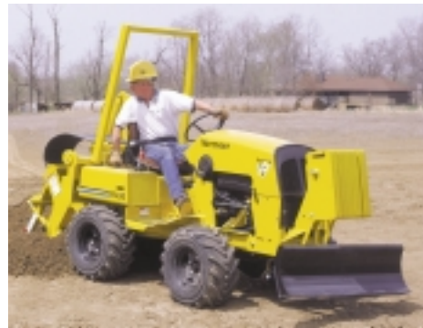
The Vermeer RT450 hydrostatic riding trencher/plow is powered by a 50-hp (37-kW) Deutz F3L2011 engine.
