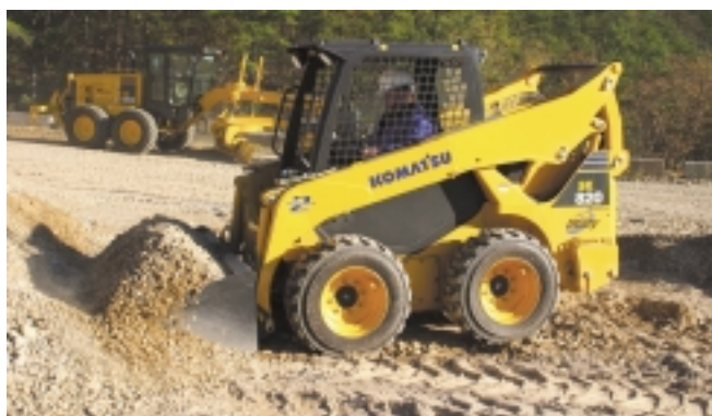
The Komatsu SK820-5 has a standard, two-speed, shift-on-the-go transmission that provides a working speed of 6.5 mph (10.5 km/h).
