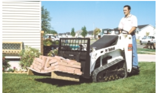
The Bobcat MT52 mini track loader, shown with a pallet fork, is powered by an 18.8-hp (14 kW) Kubota diesel engine.
