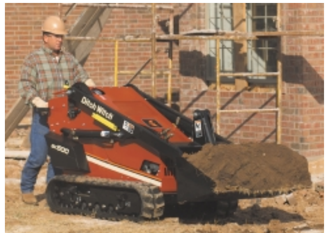
The Ditch Witch SK500 is powered by a 24-hp (18-kW) air-cooled Honda engine, and travels on rubber tracks powered by dual independent hydrostatic ground drives.
