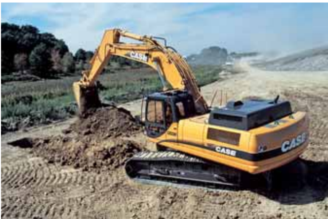
One of the enhancements to the now Tier 3-certified CX330 included increasing the strength of the front idlers by beefing up the thickness and design of the center hub and improving the track seal design for increased life.
