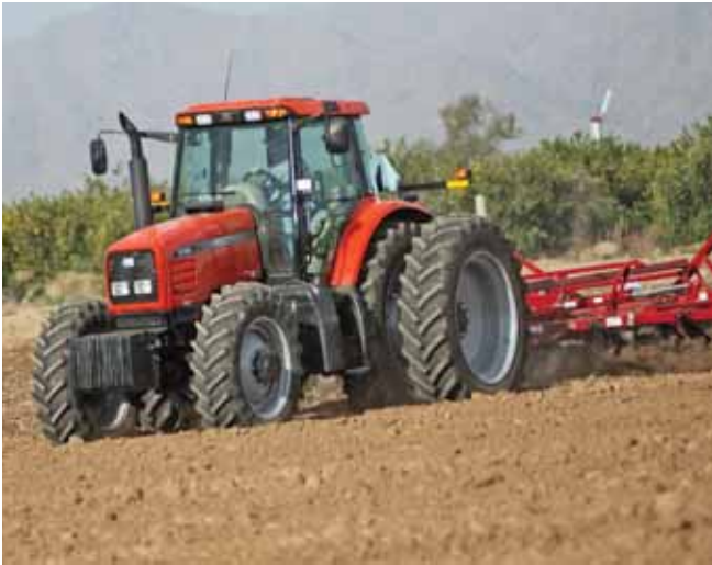
The RT155A is the most powerful model in the AGCO RT Series. AGCO says most RT buyers select the PowerMaxx CVT because of its increased efficiency and infinite speed selection.
