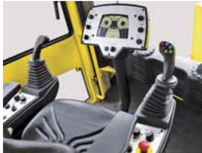
The cab of the MPH 125 features a sliding, rotating workstation; expanded leg room; and improved layout of displays and controls.
