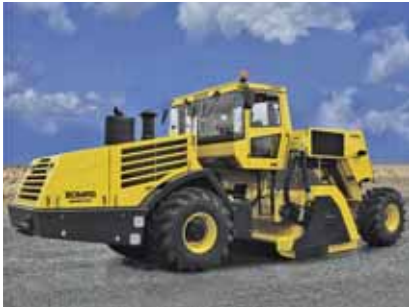
The new MPH 125 from BOMAG is designed for multi-purpose utilization in soil treatment and recycling and features a water-cooled, eight-cylinder Deutz engine.
