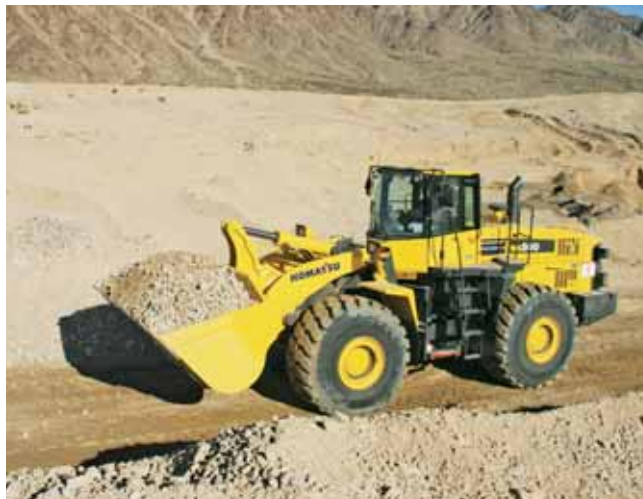
The new cab of the WA500-6 is mounted with Komatsu's unique viscous mounts to keep noise at a minimum and provide a low-vibration operating environment.
