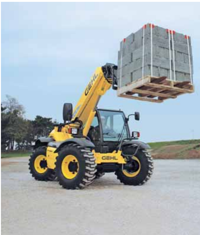
All the turbocharged models feature a vibration-insulated cab that includes a fully adjustable seat with suspension; a split-level door; rear window that opens; and front-, rear-, and roof-mounted wipers.
