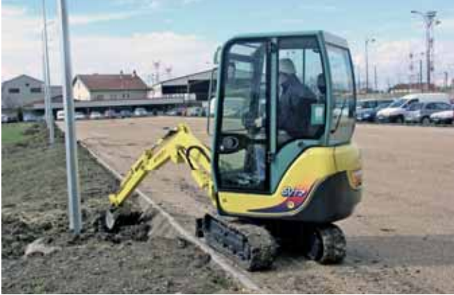
The SV17 has a dipping depth of 2400 mm (95 in), two traveling speeds, and a variable hydraulic pump. A new load-sensing hydraulic system allows for simultaneous operation of all machine functions.
