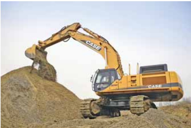
The CX700 from Case Construction Equipment has retractable side frames and an optional counterweight removal device for easier transport. It represents a new size offering for Case, fitting between the CX460 and CX800 models.
