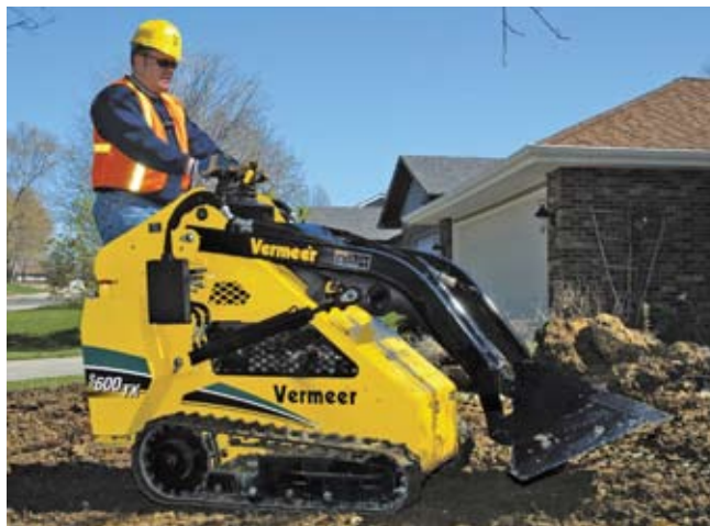
The Vermeer S600TX compact ride-on utility loader features a new Kubota engine that delivers 7% more horsepower and 11 lb-ft (15 N·m) more torque than the previous engine.
