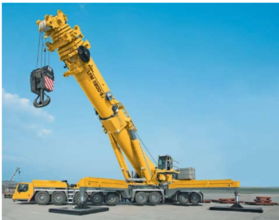
Liebherr's new nine-axle LTM 11200-9.1 all-terrain crane has a 1,200,000-kg (2,646,000-lb) load capacity and a 100-m (328-ft) boom, making it the world's strongest telescopic crane with the world's longest reach.
