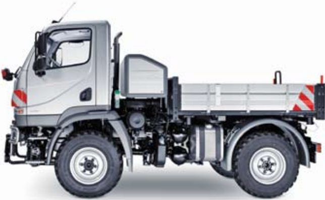
Based on the classic Unimog chassis and powertrain, the U20 features BlueTec diesel technology and a shortened wheelbase of 2700 mm (106 in).
