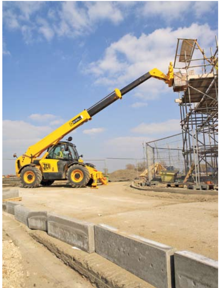
JCB's new low-boom Loadalls, including the 535-125 shown here, feature improved visibility and a tighter turning radius as well as JCB's Dieselmox engine and powershift transmission.
