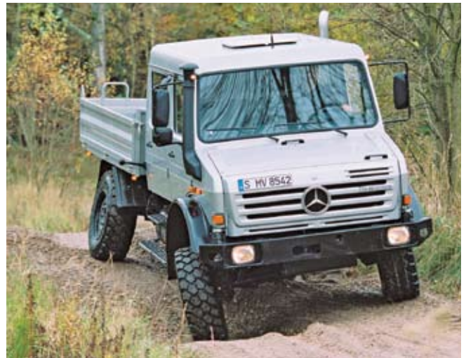
Designed for rough terrain, off-road Unimogs are available in 3250- and 3850-mm (128- and 152-in) wheelbase variants.
