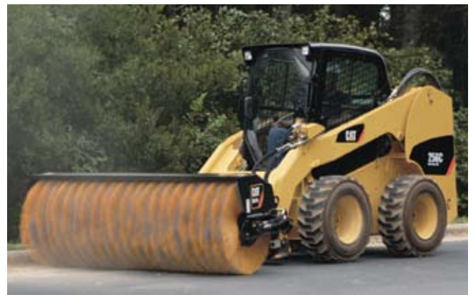
Cat's four new skid steers are all powered by the 3.3-L turbocharged Cat 3044C DIT engine and a hydrostatic drive system.
