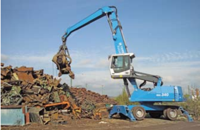
Upgrades to the Terex Fuchs MHL 340D include a larger undercarriage, larger stabilizer cylinders, an extended wheelbase, all-new dual-circuit hydraulic system, and new kinematics.
