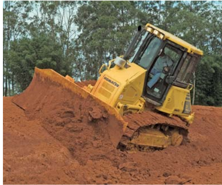
An innovative new super-slant nose design makes the D51EX/PX-22 the first bulldozer offering complete visibility of the blade's full topside and the backside of the cutting edges from the cab.
