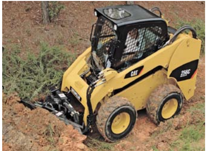
The C-Series skid steers use an electronic torque management system to maximize power to the ground; the system also enables part-throttle operation and helps to prevent the engine from stalling in tough digging and dozing applications.
