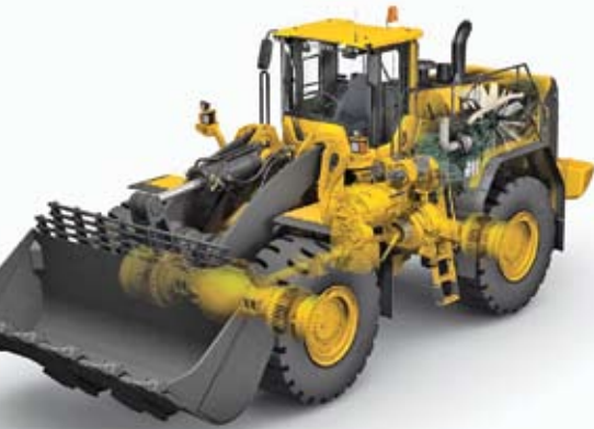
Volvo's new flagship wheel loader features the company's advanced combustion technology as well as load-sensing hydraulics and steering, an updated transmission, and an upgraded operator cab.
