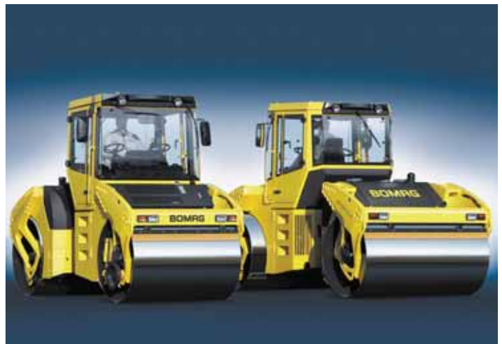
Water-cooled Deutz engines power the new BOMAG heavy articulated tandem rollers.
