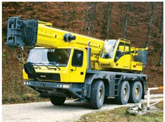
The Grove GMK3055 features a new six-section, 43 m (141 ft) MEGAFORM main boom.
