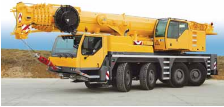
The Liebherr LTM 1090-4 mobile crane features a separate 149-kW (200-hp) diesel engine on the crane superstructure to power the hydraulics.
