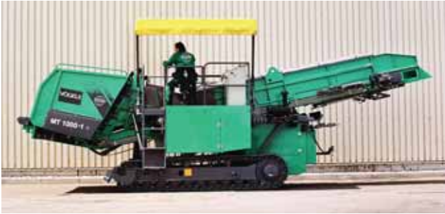
The new Vögele MT 1000-1 Mobile Feeder speeds up discharge through its belt conveyor dumping the mix from above into the paver's hopper.
