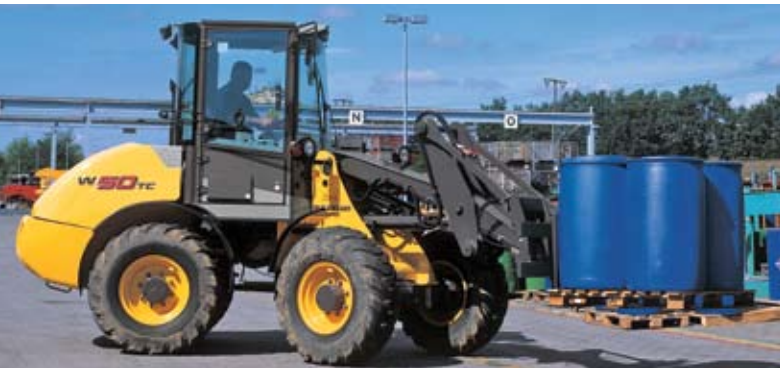
Both the W50TC and W80TC from New Holland feature all-wheel-drive with planetary axles, an oscillating rear axle, an articulated frame, outboard planetary axles, and limited-slip-differential front axle.
