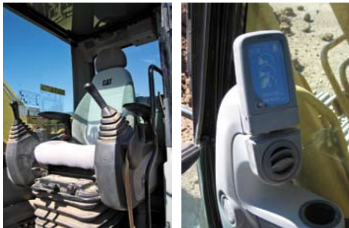
The D-Series cab is designed to be spacious, quiet, and comfortable. Cat claims that the new monitor is easier to read and navigate for both operators and maintenance technicians than the C-Series' monitor.
