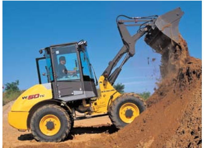
Both of the new compact wheel loaders feature a fully hydrostatic transmission with 2F/2R gears.
