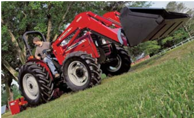
Massey Ferguson has used Perkins engines in its tractors more than 40 years, with a three-cylinder engine going in the 533, 543, and 563 (shown) and a four-cylinder engine powering the other four tractors in the new 500 Series utility tractors.
