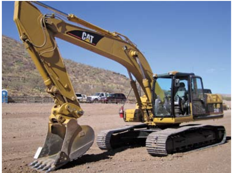
The Cat 324D is the smallest of the three new machines. It has a mass of 54,660 lb (24,790 kg) and offers 188 hp (140 kW).
