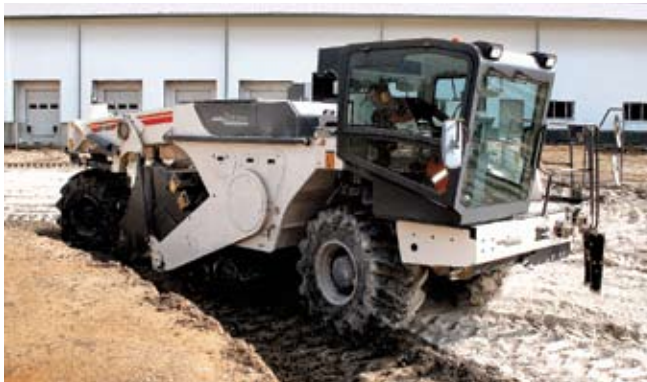
The WR 2400 stabilizes construction site terrain by blending into soil a mixture of cement and lime at a depth of 12 in (300 mm).
