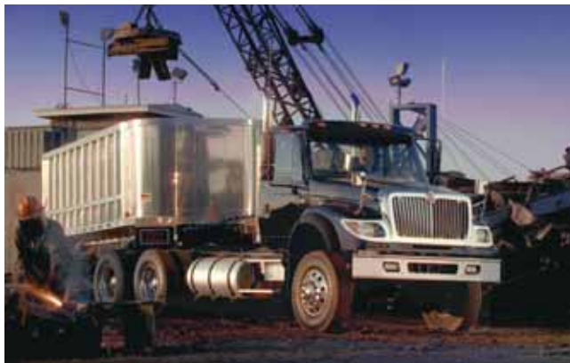
The standard engine on the International 7700 is a 305-hp (227-kW) Cummins ISM with an 1150-lb-ft (1559-N·m) rating. Engine options include an upgrade in power to a 470-hp (350-kW) Caterpillar or Cummins engine.
