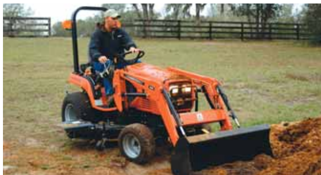
The ST22A is the first subcompact tractor from AGCO. It is powered by a 22.5-hp (16.8-kW) diesel engine.
