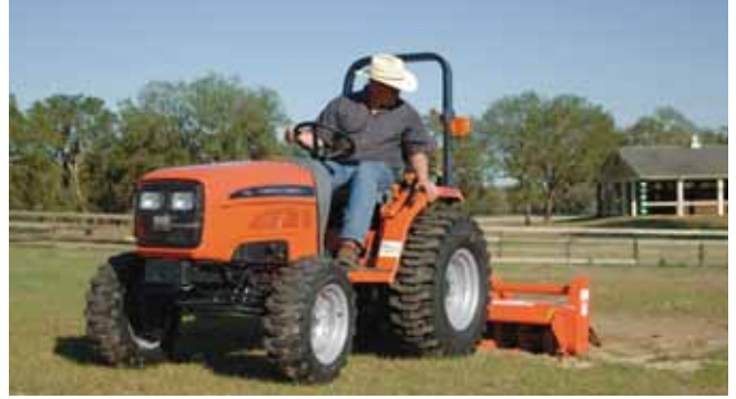
The largest of AGCO's new compact tractors, the ST33A, features a three-range hydrostatic transmission and a 33-hp (24.6-kW) diesel engine.
