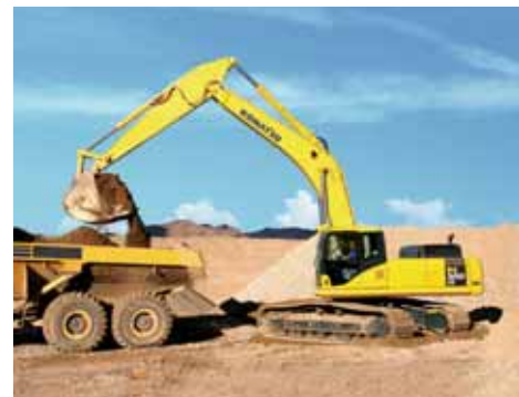
The PC300LC-7 Power Plus is powered by a turbocharged Komatsu SAA6D114E engine rated at 242 hp (180 kW).
