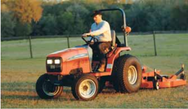
The AGCO ST24A tractor features the same engine as the ST22A but on a chassis built for heavier loads.
