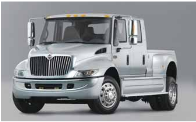
The International RXT is a 22-ft (6.7-m) commercial pickup truck with (depending on configuration) a payload of up to 8 ton (7.3 t) and towing capacity of up to 12 ton (10.9 t). It features commercial hydraulic brakes for stopping large loads or trailers.
