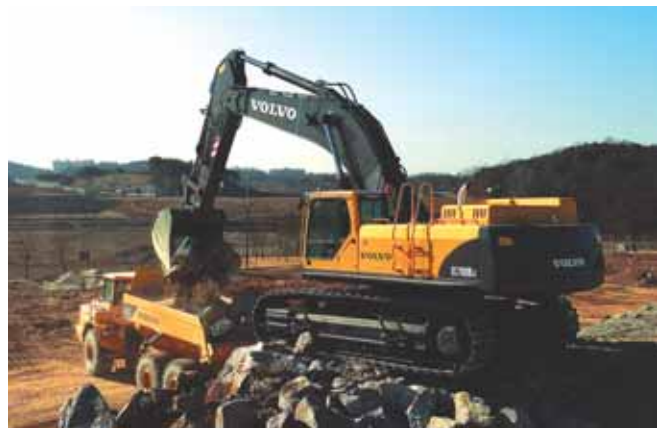
Power for Volvo's new EC700B excavator comes from the Volvo D16C EAE3, with a gross output of 464 hp (346 kW) at 1800 rpm. The engine uses the new Tier 3-compliant Volvo Advanced Combustion Technology.
