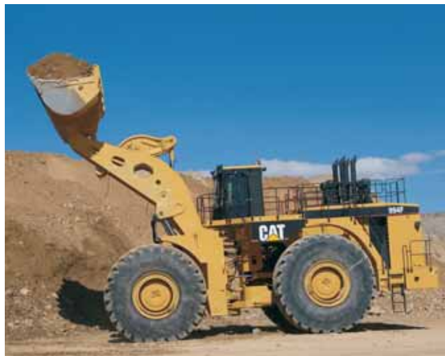
Caterpillar's 994F wheel loader is powered by the Cat 3516B HD EUI engine that delivers 1577 gross hp (1174 kW). Net power is 1429 hp (1065 kW).
