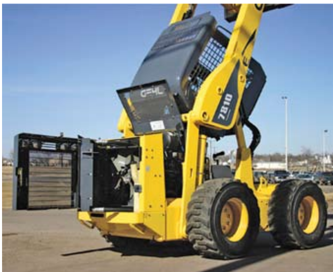
The cab of Gehl's new 7810E can be pivoted up and out of the way for maintenance via a built-in hydraulic pump or with an optional electric pump.
