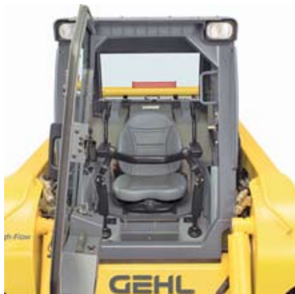
Plenty of head, shoulder, and leg room is available in the 7810E's cab, as well as plenty of control choices, including joystick, dual-hand, hand-foot, and T-bar.
