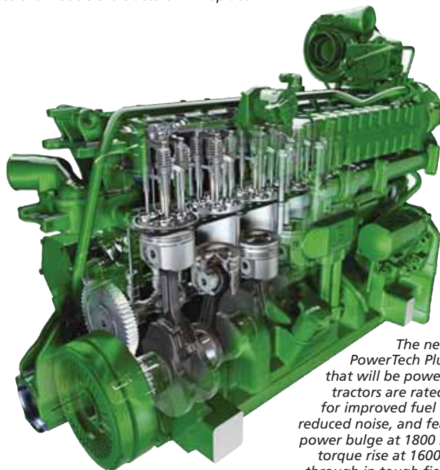
The combination of its own engines, cooling systems, and other tractor elements allowed Deere engineers to integrate technology into the 8030 Series tractors that it says results in a 2 to 5% reduction in fuel consumption compared to the models the tractors will replace.
