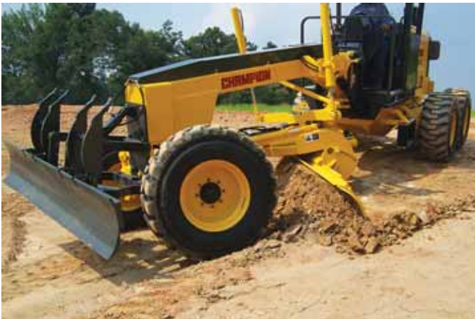
The C80/C86 C Series from Champion Motor Graders features redesigned front axle components, the moldboard and blade lift arrangement, and the articulation cylinder.
