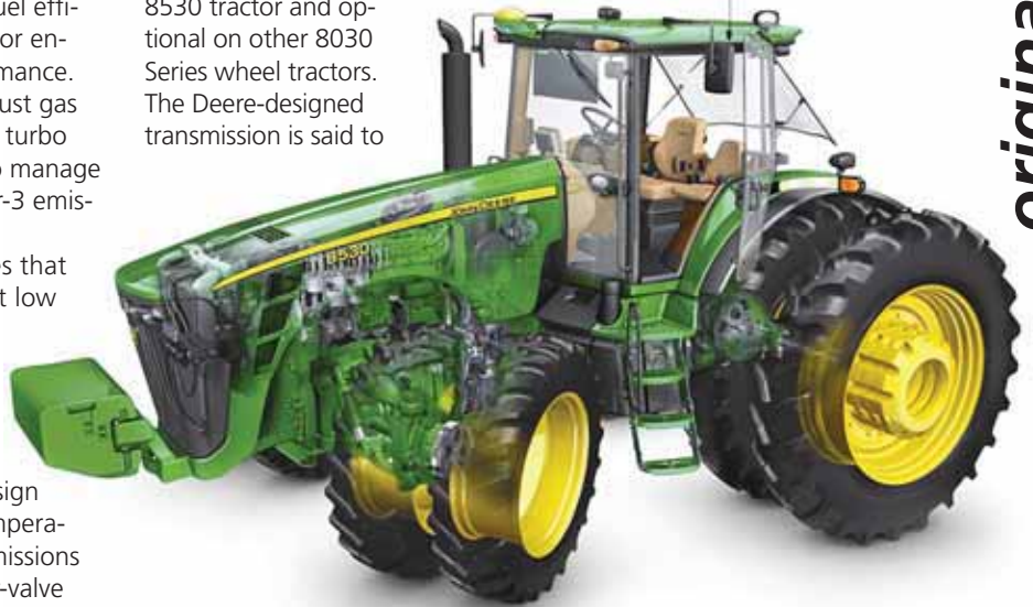
The combination of its own engines, cooling systems, and other tractor elements allowed Deere engineers to integrate technology into the 8030 Series tractors that it says results in a 2 to 5% reduction in fuel consumption compared to the models the tractors will replace.
