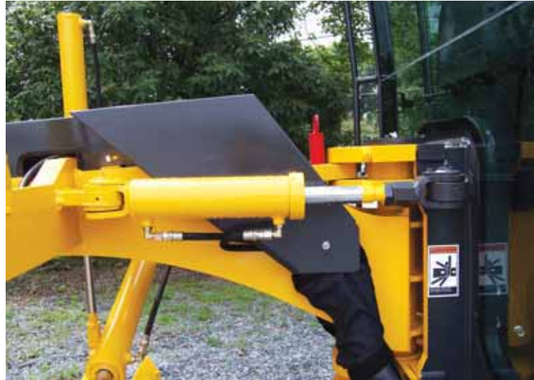
Champion took out the replaceable ball joints and engineered in clevis-style mountings for greater strength at the articulation cylinders.
