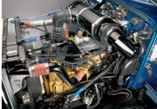
The Caterpillar C9 engine, which reduces mass by 780 lb (354 kg) when compared with the C11, is available with power ratings of 335 and 350 hp (250 and 261 kW) for the Peterbilt Model 357-115 and Model 357-111.
