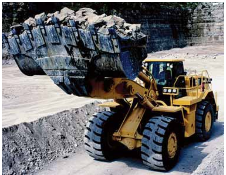
Biggest of Cat's new line is the 988H wheel loader, which features a new Cat C18 engine rated at 354 kW (475 hp) net.
