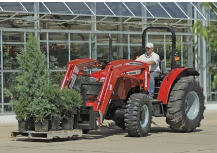
The hydraulics on the 3600 tractors feature an open center system that is capable of supplying 15.8 gal/min (60 L/min) to the rear remotes.
