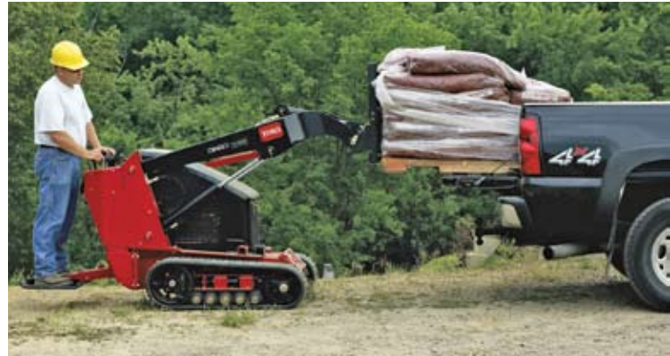
The TX Platform attachment offered for three of Toro's Dingo models is expected to decrease operator fatigue, especially during applications that require extensive hauling for long distances.
