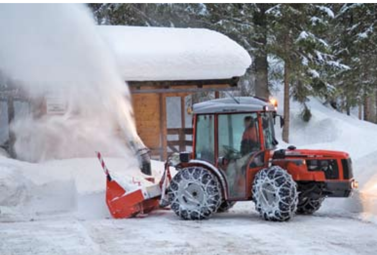
The hydrostatic transmission on the new HTX 9400 tractor from Antonio Carraro offers an infinite range of speeds in both drive directions.
