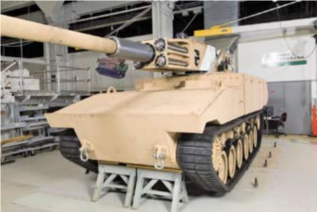
The Firing Platform features an ultra-lightweight, 38-caliber 155-mm howitzer integrated with a fully automated ammunition handling system.
