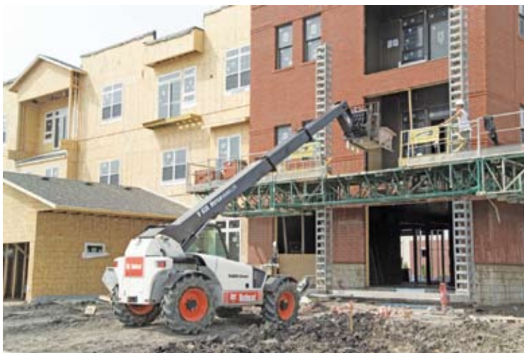
The V638 has a maximum load capacity of 6700 lb (3040 kg) and a maximum lift height of almost 39 ft (12 m).
