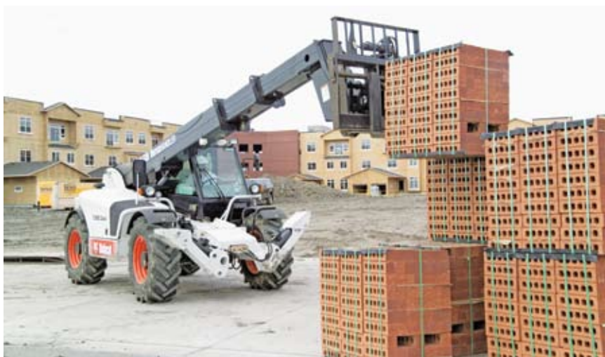
Bobcat says it mounted the engine of the V638 on the right-hand side to provide operators better visibility to the sides and rear of the machine.
