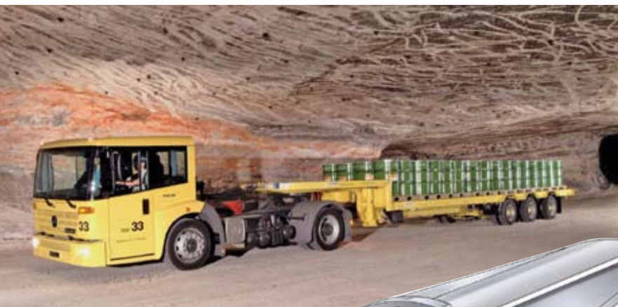
Mercedes-Benz' Econic, used to transport industrial waste in the Herfa-Neurode salt mine in Germany, is equipped with an Allison 3060 fully automatic transmission.
