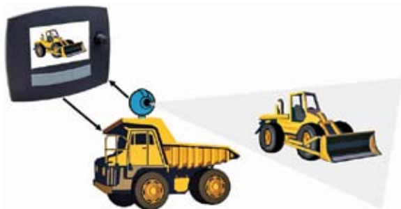
TTControl's camera vision system was designed to avoid dangerous situations on a job site that are caused by bad or limited view for the operator.
