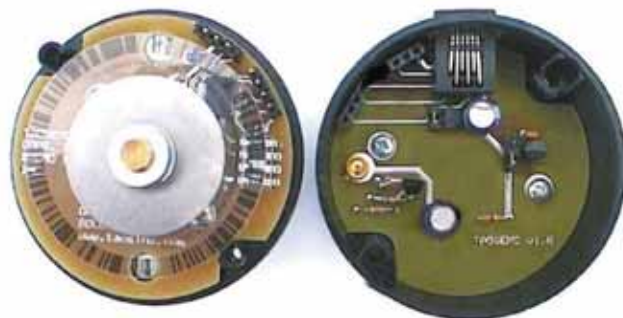
The TAOS/Microchip Technology optical rotary encoder was shown as a demonstration device during Convergence.
