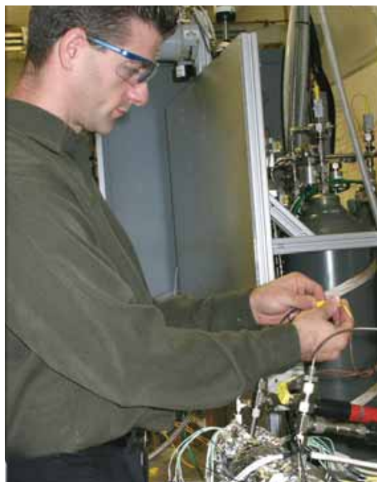
Recharging of the hydrides and release of the hydrogen from metal hydrides such as sodium alanate requires heat, which can reduce overall fuel economy. Sandia National Laboratories engineer Terry Johnson sets up a test apparatus that, when verified, will generate external heat that improves the overall energy density compared to traditional heat sources. (Photograph courtesy of Bud Pelletier.)
