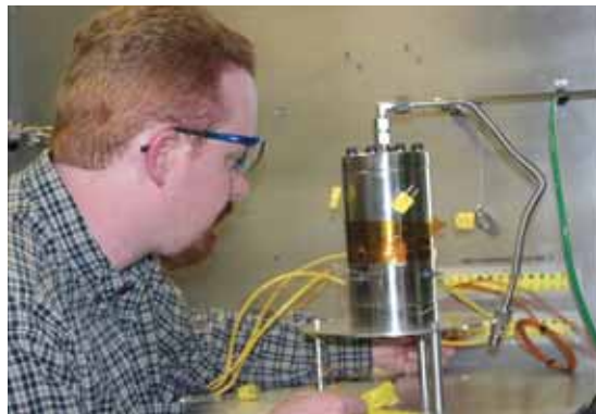
A critical aspect of hydride storage tank development is the act of recharging and discharging hydrogen. Here, Sandia National Laboratories engineer Mark Zimmerman integrates a hydride bed with temperature-monitoring sensors. (Photograph courtesy of Bud Pelletier.)
