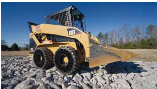
A production-ready skid-steer loader application for Michelin's Tweel is possible in a couple of years while active research projects are under way with the military.
