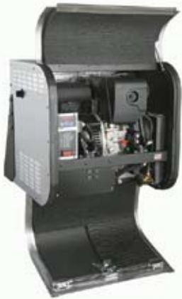
The APU comes standard with a digital controller that will allow drivers to start and stop the generator from inside the cab.
