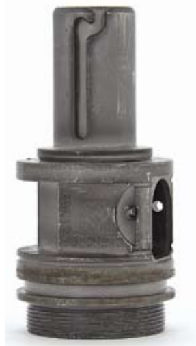
Timken engineers developed a hot-rolled temper process to produce steel that can be more easily machined for a Bosch diesel fuel injector used on truck engines.
