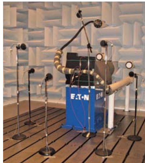
Easton's new sound chamber will enable it to validate models and benchmark the competition—capabilities it considers to be critical to support its emphasis on NVH modeling and simulation efforts.
