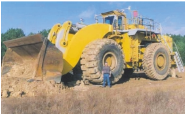
Because the loader has electric drive and drive-by-wire, susceptibility of the control systems to outside interference is of critical importance for safe operation.
