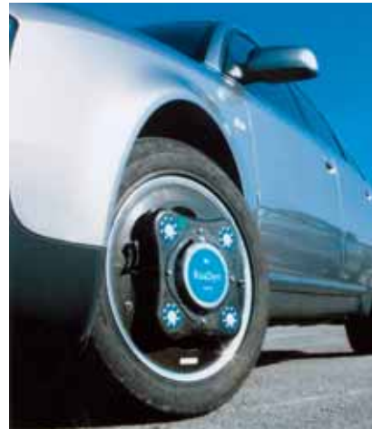
The RoaDyn wheel-force measuring system does not affect performance, braking, or steering.
