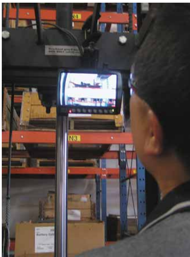
The vision system envisioned by Raymond would use cameras and/or lasers mounted on the fork carriage to make it easier for operators to position the forks for put-away and retrieval of loads.
