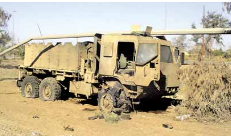
The crew walked away from this truck fitted with a Radian Armored Cab Kit after it was hit by a suicide car bomb.
