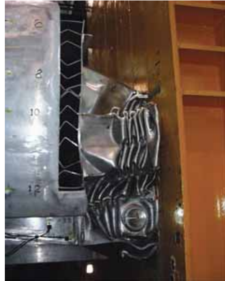
Alcan MTS built a full-scale prototype of the crash zone, upon which quasi-static physical testing verified the analytical predictions from ABAQUS.
