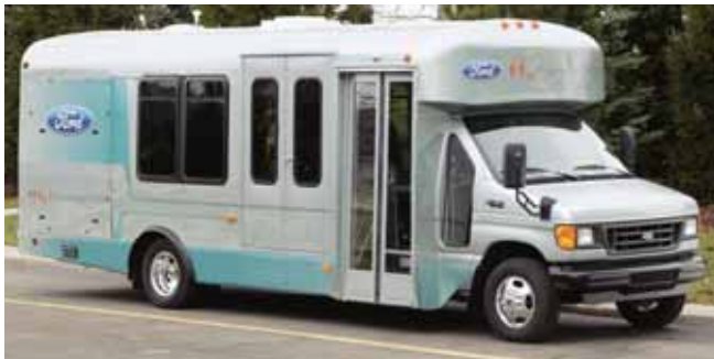
Ford's 2006 E-450 shuttle bus for airline ground support will be powered by the company's hydrogen-powered V10 internal-combustion engine, which is a modified version of the company's Triton engine.
