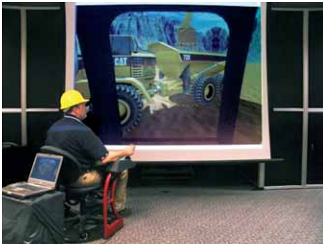
Cat's Virtual Training System consists of software, a chair base assembly, and joystick control module. The simulated image can be viewed on a computer screen or connected to a LCD television or projection screen.
