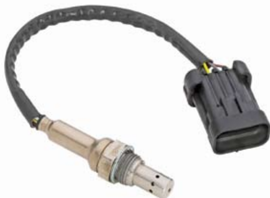
For use in selective catalytic reduction systems, Delphi's ammonia sensor measures ammonia levels in the exhaust gas, which allows for the precise dosing of urea.
