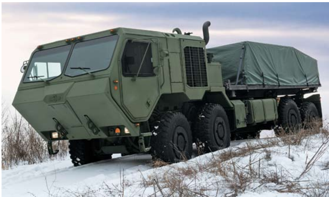
Oshkosh's third-generation Heavy Expanded Mobility Tactical Truck features a diesel-electric drive system that makes use of copper rotors for the ac induction motors.
