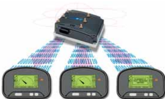
In this depiction of the data stream, Curtis Instruments' model 1238 motor controller transmits battery state-of-charge information to enGage IV via CAN bus (A, left), the vehicle operator pushes a front-panel button to initiate a CAN request to the 1238 for diagnostic information (B, middle), and the 1238 transmits pages of diagnostic history that the operator can scroll through using front-panel buttons (C, right).
