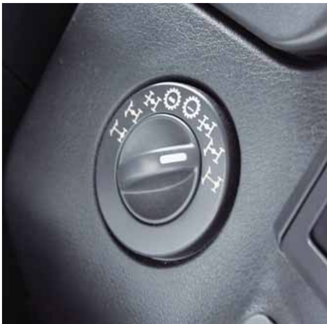
For safety and ease of use, MAN controls the inter-axle and transverse differential locks in a logically correct sequence using a rotary switch.
