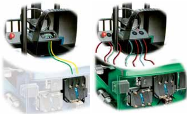
Distributed processing (left) allows simplified vehicle design and wiring by using the two-wire CAN bus to communicate all vehicle information between the enGage IV and model 1238 processing hubs, unlike the multitude of wires it took on older systems (right).
