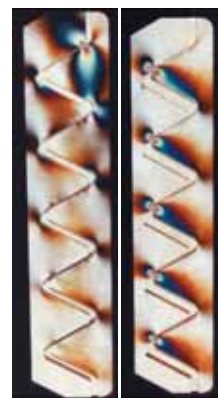
This photoelastic comparison illustrates how the load carried by each engaged thread is more uniform with a Spirallock thread (right) compared to a conventional one.
