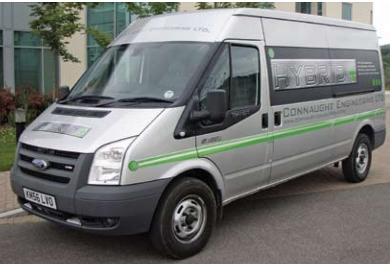
Connaught's "bolt-on" Hybrid+ system, the first application of which is in Tesco Ford Transit cargo vans, takes drive from the lower front pulley of the vehicle's engine.
